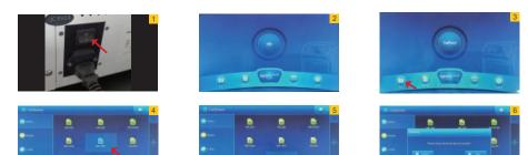
1. Turn on the **'power switch**' located on the right rear of the GENTi<sup>™ 32</sup> Advanced Automatic Extraction System.
